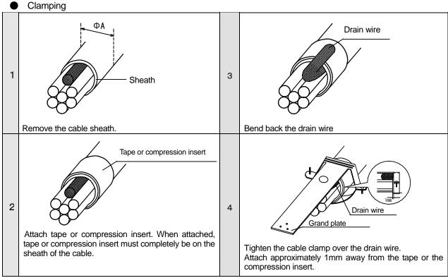
\* Compression insert should only be attached before soldering the cable to the connector
