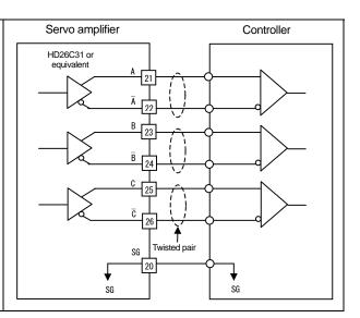
Absolute position data output circuit (Model number : TS1\*\*\*AF) [output circuit : line driver]
