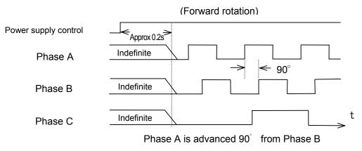
After turning ON the system, the power supply is not fixed for about 0.2 sec.
