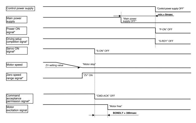
The signal of sign (\*) can be allocated to general-purpose output OUT1 to OUT5.
