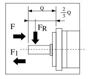
• The permissible loads during operation were determined corresponding to the revolution rate of the motor and the load being applied to the output shaft of the motor and in consideration the service life of the bearing and shaft strength.
