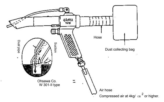
Fig.12 Example of a dust collector. (an inhale type)
