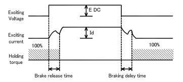
The brake release time and braking delay time refer to those mentioned in the above tables.
