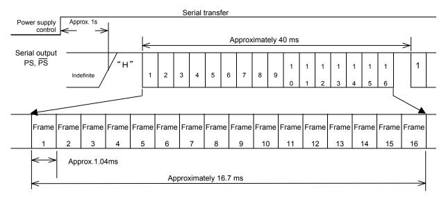
Selection value 02:\_Encoder\_Signal Encoder signal direct output
