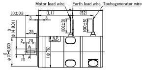
Tochogenerator wire Brake lead wire Earth lead wire Motor lead wire T720BT-012, T730BT-012 (4<u>3.5</u>) <u>30±0.8</u> (L1) (52) 8 3 1000±50 1000±50 1000±50 14-0.01 25 20 70-0.030 в 5 SECTION A-A
