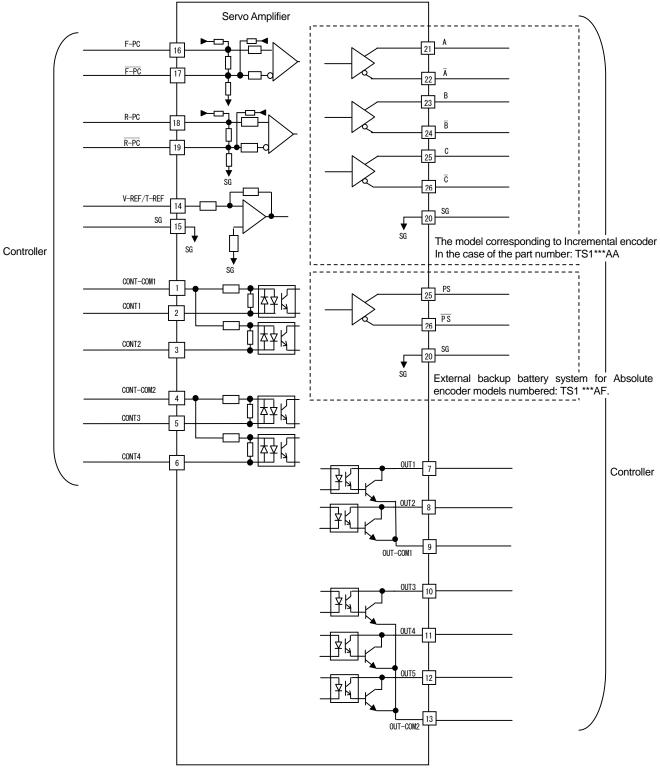
Connection example with analog input circuit
