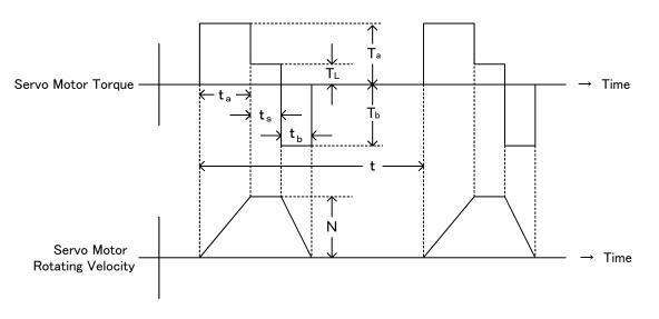
If the operating cycle is considered as 't', the usable range can be determined as follows:
