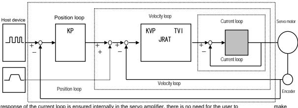
The response of the current loop is ensured internally in the servo amplifier, there is no need for the user to additional adjustments.
