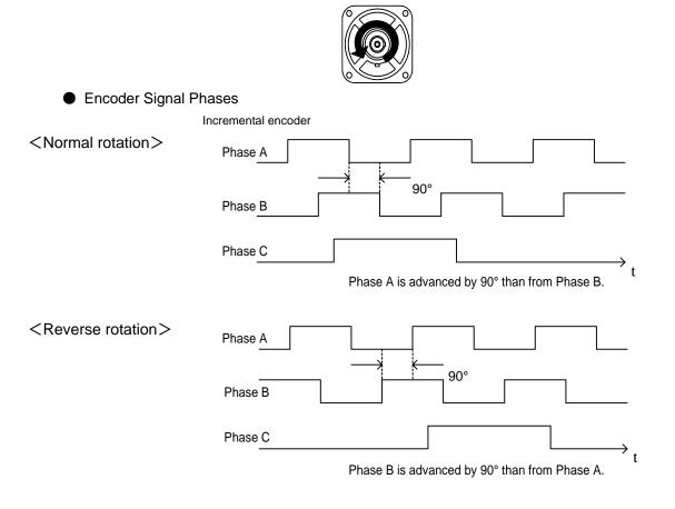
When the C-Phase is high, both A- and B- Phases cross the low level, once every revolution.
