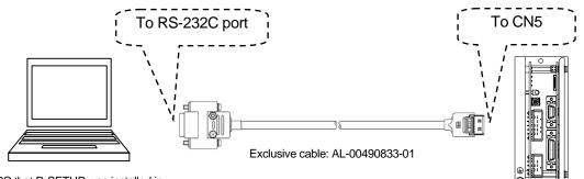
The PC that R-SETUP was installed in.
