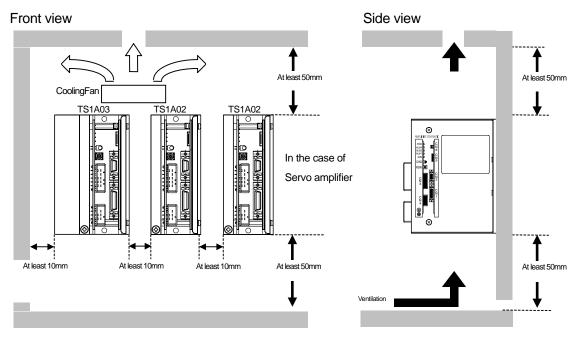
Please note the following regarding the installation location and mounting method for the servo motor.
