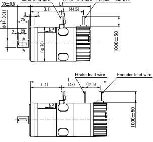
Earth lead wire Encoder lead wire
